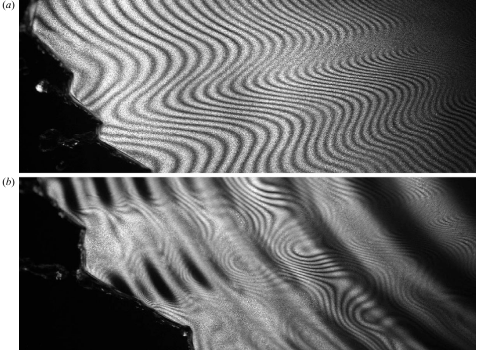
FIGURE 19. Thickness field revealed through laser interference of (a) a smooth and free liquid sheet exhibiting smooth azimuthal thickness modulations, and (b) with forced surface undulations where the transverse modulations of the thickness are amplified. Both pictures cover the same field.
