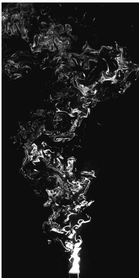
FIG. 1. A snapshot of a dispersing plume made by the injection of a dye through a small tube of d=8 mm in diameter on the axis of a larger turbulent jet whose integral scale is L=8 cm at the injection location: Re=u'L/\nu=10^4 .
