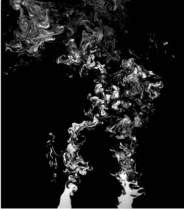
FIGURE 2. Two sources discharging in a turbulent medium in which they mix. Their separation is of the order of the local integral scale L .
