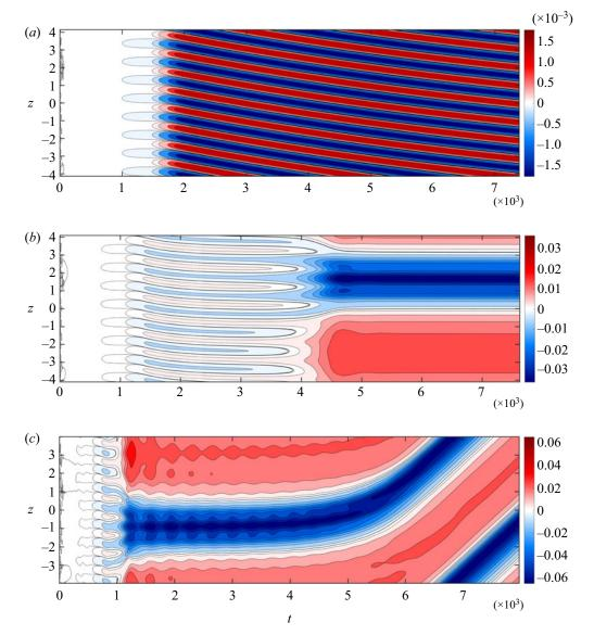
Figure 3. Hovmöller diagrams of the horizontally averaged streamwise velocity fluctuation  $\langle u - U_0 \rangle_H$ , computed in the (t, z)-plane. Positive (negative) values are displayed in red (blue). The area of constant colour on the left of each plot represents the exponential growth of disturbances. Reynolds numbers are (a) Re = 550, (b) Re = 580, and (c) Re = 700.
