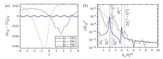
Figure 4. Each curve is computed at the latest time of simulation in figure 3, once the solution has converged. (a) Horizontally averaged streamwise velocity fluctuations as a function of the vertical coordinate. (b) Spectral energy in Fourier space of the averaged velocity profiles from (a). The principal amplitude peaks are displayed with vertical lines and labelled with their associated representation defined in (4.5).
