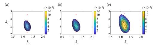
Figure 1. Growth rate contours in the  $(k_x, k_z)$  space from the linear stability analysis of (3.2) at Fr = 2, Sc = 1 and over different Reynolds numbers: (a) Re = 550, (b) Re = 580, (c) Re = 700. Red crosses correspond to the discretized modes present in our DNS domain (cf. § 4). White regions correspond to negative growth rates, i.e. stability.
