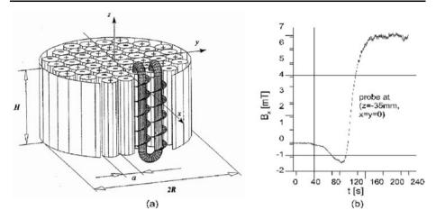
**Fig. 9** The Karlsruhe dynamo experiment. (a) Central part of the facility. The module consists of 52 spin-generators, each containing a central tube with non-rotating flow and an outer tube where the flow is forced on a helical path. (b) Self-excitation and saturation in the Karlsruhe dynamo experiment. Hall sensor signals of  $B_X$  in the inner bore of the module. Figure taken from Stefani et al. (2008)
