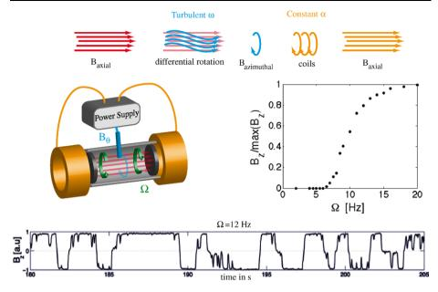
**Fig. 7** The Bullard von-Kármán dynamo. (top): Principle of dynamo feed-back loop with actual implementation (middle left). The mid-right curve is the bifurcation curve of the self-sustained magnetic field as the rotation rate of the impellers increase. The bottom figure shows an example of time signal, with reversals of the dipole field, figure from Bourgoin et al. (2006)
