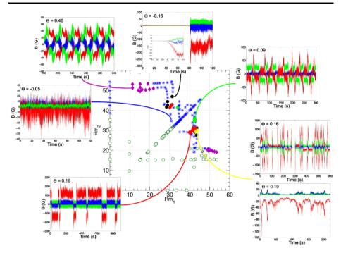
**Fig. 12** Dynamical regimes observed in the von Kármán sodium experiment when the impellers driving the flow rotate at varying rates: the coordinates in the main plot are the magnetic Reynolds numbers built from the velocity of each impeller. The *insets* give examples of time signals of the 3 components of the magnetic field recorded in the mid-plane of the cylinder. Figure extracted from data in Monchaux et al. (2009)
