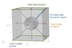
IFluid domain: newtonian,  $\rho$ =997 kg/m<sup>3</sup>,  $\mu$ =885× 10<sup>-4</sup> kg.m<sup>-1</sup>.s<sup>-1</sup>
