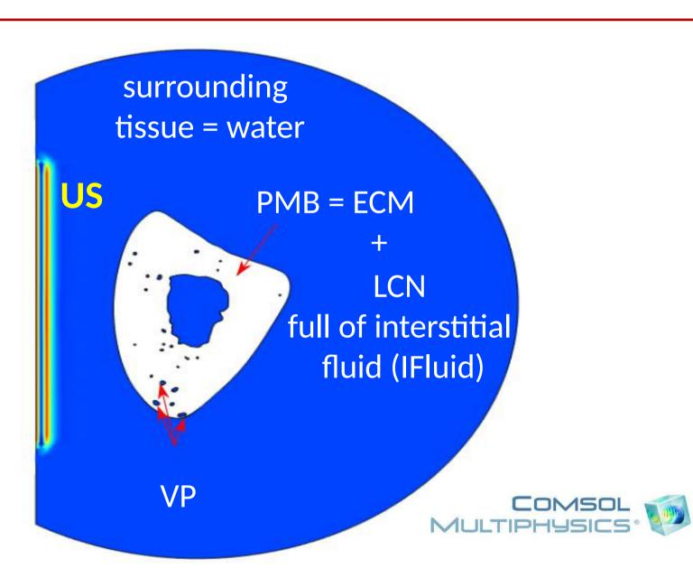
US stimulation frequency = 1MHz, pressure = 67kPa, duty cycle = 20%, pulse duration = 1ms  $\emptyset$ transducer = 20mm
