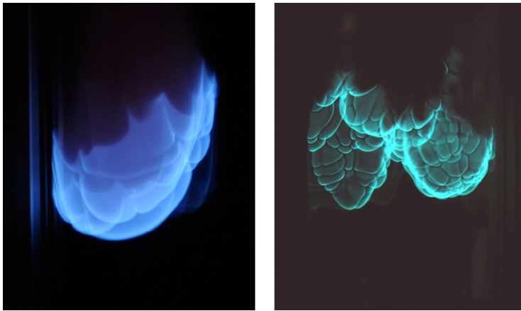
Fig. 6 Rich methane-air (left: \phi = 1.3 ) and propane-air flame (right: \phi = 1.4 ) in a tube 140 mm inner diameter.
