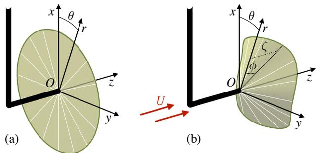
Figure 1. Experimental setup. A flexible circular plate is clamped onto an elbow (a). When placed in a uniform water flow of velocity  $U$ , the plate deforms (b). The function  $\phi(\theta)$  describes the d-cone deformation of the plate.
