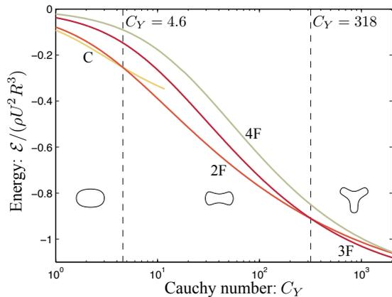
Figure 4. Energy as a function of the Cauchy number for the modes C, 2F, 3F, and 4F. These energies are found by minimizing the total energy  $\mathcal{E}$  when the deformation amplitude is varied. The calculation for mode C is stopped when the radius of curvature reaches  $2R/\pi$ .
