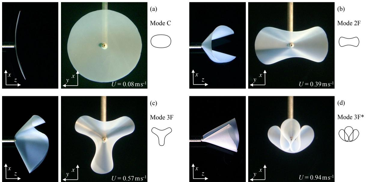
Figure 2. Draping modes of a circular plate of radius  $R = 0.05$  m. When the flow velocity is gradually increased, different draping patterns become visible starting from “mode C”, a cylindrical mode (a), to “mode 2F”, a two-fold conical mode (b), “mode 3F”, a three-fold mode (c), and eventually “mode 3F\*”, a bent three-fold mode (d).
