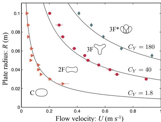
Figure 3. Morphological diagram in the  $U$ - $R$  plane. The symbols mark the transitions, as the flow velocity is increased, between the different modes pictured. The error bars on the triangles, associated to the C-2F transition, correspond to a continuous transition, while the error bars of the 2F-3F transition (circles) correspond to an intermittent coexistence of the two modes. The solid lines are iso-values of the Cauchy number as defined in Eq. (3).
