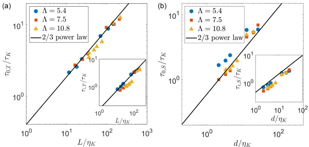
FIG. 7. Evolution of the zero-crossing time for (a) tumbling rate as a function of the normalized fiber length ( $L/\eta_K$ ) and (b) spinning rate as a function of the normalized fiber diameter ( $d/\eta_K$ ). Each inset shows the evolution of the integral correlation timescale for the respective component of rotation.
