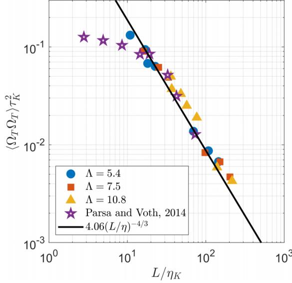
FIG. 3. Dimensionless variance of tumbling rate of inertial fibers against dimensionless fiber length. The prefactor in the  $-4/3$  power-law is obtained from a least-squares fit of the experimental data.
