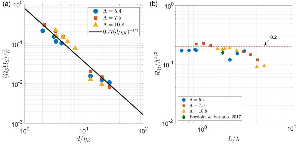
FIG. 5. (a) Dimensionless variance of spinning rate as a function of the dimensionless fiber diameter and (b) a compensated ratio between the variances of the spinning and the tumbling rate ( $\mathcal{R}_\Omega/\Lambda^{4/3}$ ) against fiber length  $L$  normalized by Taylor length  $\lambda$ .
