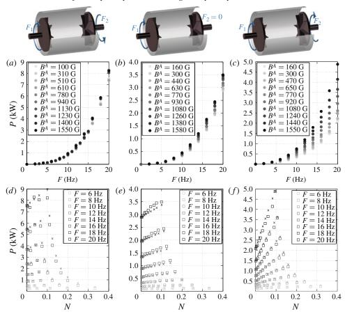
FIGURE 3. (Colour online) Evolution of the injected power as a function of the rotation rate F(a-c) and as a function of the interaction parameter N(d-f): measurements  $(\Box)$  and estimation  $(\times)$ , see § 4.2. The applied magnetic field is perpendicular to the axis of rotation. The three investigated flows are: counter-rotating flow (a,d), one-disk flow (b,e) and corotating flow (c,f).
