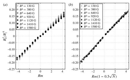
FIGURE 6. Evolution of the azimuthal induced magnetic field from an axial applied magnetic field with a counter-rotating flow, as a function of (a) the magnetic Reynolds number Rm and (b) an *effective* magnetic Reynolds number  $Rm(1 - \alpha \sqrt{N})$ .
