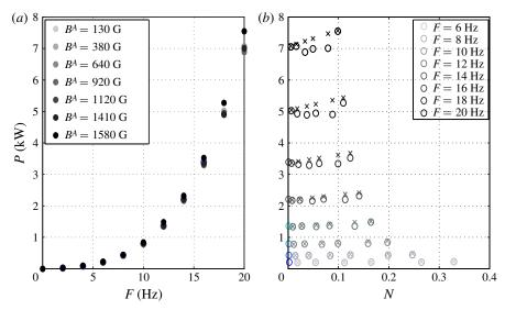
FIGURE 4. (Colour online) Evolution of the injected power for the counter-rotating flow with an axial applied field as a function of the rotation rate (*a*) and the interaction parameter (*b*): measurements ( $\circ$ ), estimation ( $\times$ ), see § 4.2.
