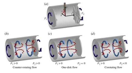
FIGURE 1. (Colour online available at journals.cambridge.org/flm) (a) Geometry of the experimental setup (see details in the text), and coordinate system used throughout the text; the magnetic probe shaft is along the y-axis. (b) Counter-rotating (s2t2) flow: two counter-rotating toroidal cells (plain arrows) and two poloidal cells (dashed arrows). (c) One-disk (s1t1) flow: one toroidal cell and one poloidal cell. (d) Corotating (s2t1) flow: one toroidal cells.
