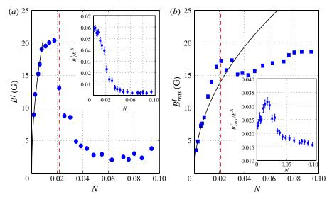
FIGURE 7. (Colour online) Evolution of the axial component of the induced magnetic field measured in the mid-plane as a function of N: (a) time-averaged value; (b) standard deviation. The disks rotate at 12 Hz in opposite directions and the applied magnetic field is transverse. Insets show value normalized by the applied magnetic field. The solid line corresponds to a fit of the experimental measurements in the hydrodynamic regime and the dashed line corresponds to  $N = B^I/B^A$ .
