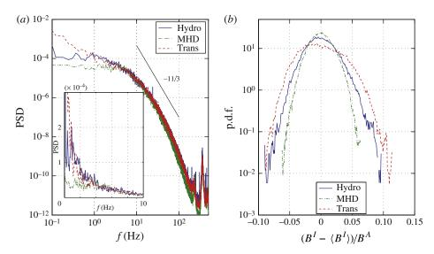
FIGURE 9. (Colour online) (a) Power spectral density of the normalized induced magnetic field with a transverse applied magnetic field and a counter-rotating flow, F = 12 Hz, for three values of the applied magnetic field:  $N = 1.5 \times 10^{-3}$ ,  $B^A = 150$  G, (plain);  $N = 1.4 \times 10^{-2}$ ,  $B^A = 460$  G (dashed) and  $N = 6.2 \times 10^{-2}$ ,  $B^A = 970$  G (dashed dot). (b) Corresponding centred probability density functions.
