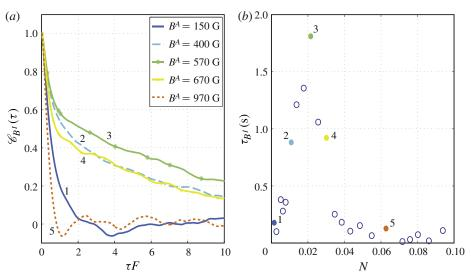
FIGURE 8. (Colour online) (a) Correlation function  $\mathcal{C}_{B^{I}}(\tau)$  of the induced magnetic field for different applied magnetic fields. (b) Correlation time of the induced magnetic field as a function of the interaction parameter. Colours correspond to values at which the correlation function evolution is displayed in (a).
