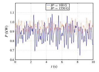
FIGURE 2. (Colour online) Time evolution of the power consumption, measured from the output of the motors' electric power supplies. Counter-rotating case at 10 Hz with an applied magnetic field  $B^A = 100$  G (solid line) and  $B^A = 1550$  G (dashed line).
