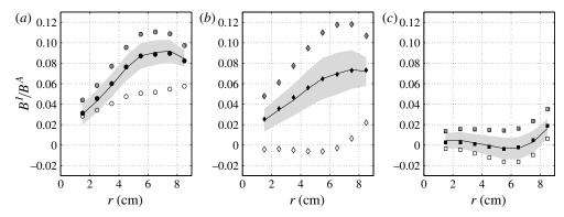
FIGURE 10. Instantaneous profiles of the axial induced magnetic field in the mid-plane: (a)  $B^A = 150$  G, hydrodynamic regime; (b)  $B^A = 520$  G, transition regime; (c)  $B^A = 1200$  G, MHD regime. The black symbols correspond to the time-averaged induction profile. The furthest profiles from the mean values are represented by grey symbols (greater than the mean) and open symbols (smaller than the mean). The grey area corresponds to the standard deviation of the profile.
